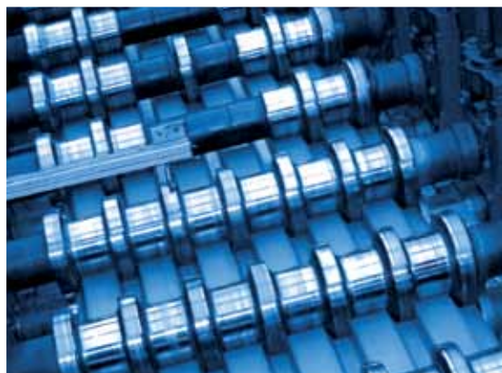
Metal Dek products are rolled formed on form rollers at the company's metal deck facilities in Memphis, TN, Phoenix, AZ, Terrel, TX, and Harrisburg, VA.
